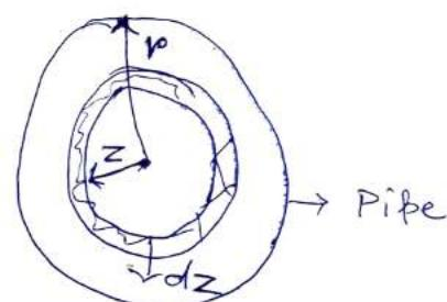
Now if we consider it as liquid flow, the liquid which is in contact with the pipe is stationary and the velocity of the layers increases with increasing distance from the surface. That means the velocity of the layer which is in the middle is maximum. If the velocity gradient is  $\frac{dv}{dr}$  and area of contact is A then the internal frictional force(f) which is dragging the liquid to flow, as per Newton
