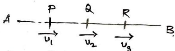
When the velocity of the particles in a liquid flow-line exactly the same in ~~each~~ points in its path of movement both in magnitude and direction. It is not necessary for all the particles, the velocity to be constant or same at its whole path.
