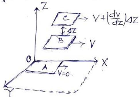
Let the gas is flowing in layers parallel to XY-Plane. Let A, B and C are such layers. Layer A is in contact with XY-Surface. So the Velocity would be zero at that plane. with increasing distance from XY- Plane in the Z-direction, the velocity of the layers will also increase.
