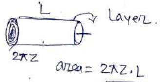
For the steady rate of flow, this frictional force is exactly the same with the driving force  $\pi z^2 (P_1 - P_2)$  where  $(P_1 - P_2)$  is the pressure difference of the two ends of the pipe.
