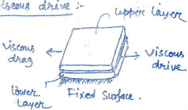
The viscous drag is a kind of friction or fluid resistance, acting relatively to the opposite of motion of fluid. This can exist between two layers of a fluid and a solid surface. The drag force is proportional to the velocity for the laminar flow and squared velocity for a turbulent flow.
